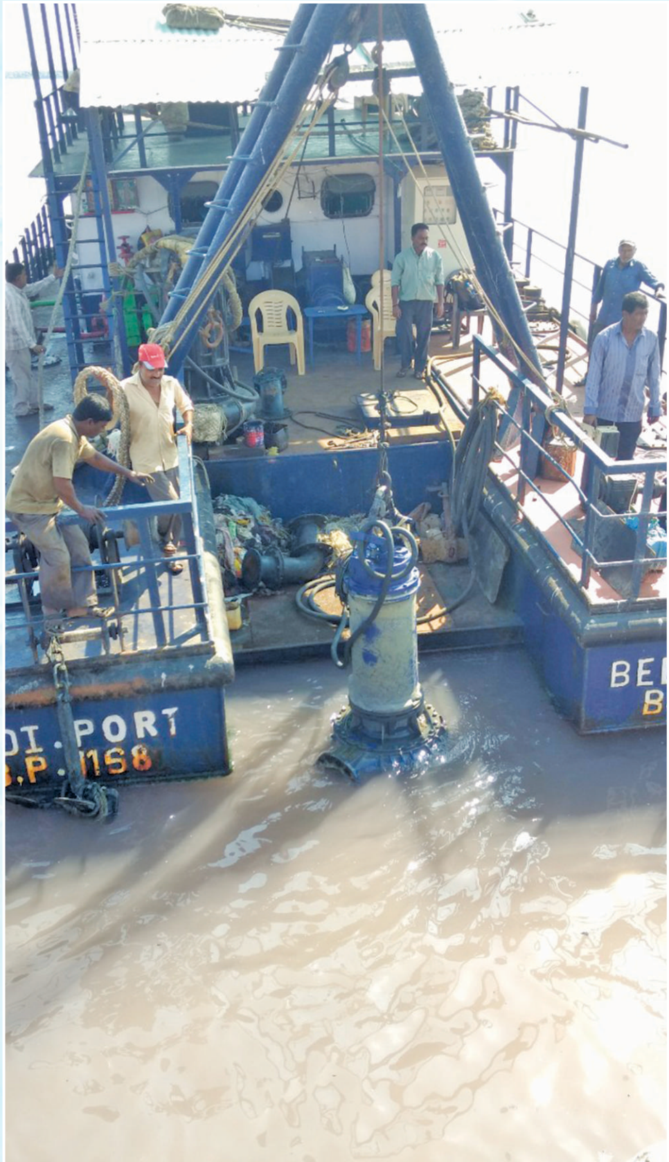
An Aqua ADS Submersible Dredging pump being lowered for dredging
